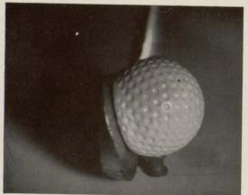
Fig. 5. High-speed photograph, 1/75,000th second. Golf ball photographed at moment of impact by mashie. Note flattening of ball. High intensity spark discharge automatically fired by interrupted light beam and a photo-electric cell. Output of cell amplified sufficiently to trip the spark. Photograph by H. E. Edgerton and K. J. Germes-Lausen, Massachusetts Institute of Technology. Courtesy Arthur D. Little, Inc., Cambridge, Mass.
