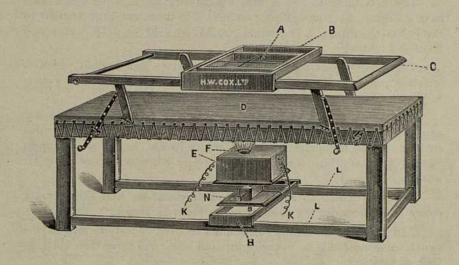
Remove the plate carrier from the frame and lower the latter to enable the patient to be placed easily on the couch.
