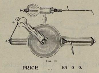
The anode of an ordinary Tube is soon destroyed if used for any length of time with an Electrolytic Interruptor, in consequence of the great heat.
