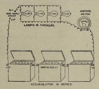
The accumulators should be connected together in series, *i.e.*, the positive terminal of one cell is connected to the negative terminal of the next cell, and so on, leaving one positive and one negative unconnected at the ends. The positive terminal is marked thus + or painted red, and the negative terminal thus — or painted black. The two end terminals
