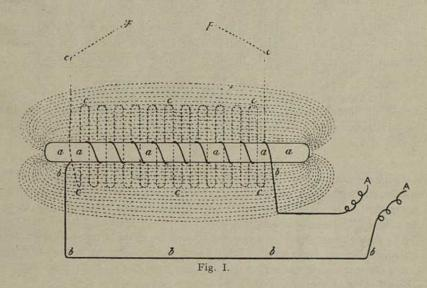
The secondary coil, which consists of many thousands of yards of very fine insulated copper wire, is wound round the core and primary circuit in such a manner that it is continually passing through the magnetic field.
