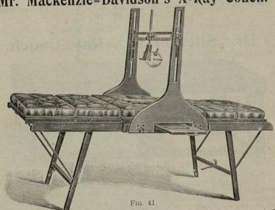
Although Couches of the type first described have been generally adopted, that here shown can scarcely be surpassed for precise localisation and stereoscopic purposes. It will be seen that the Tube is placed above the patient, and the plates underneath him. The latter are changed by means of a slide inserted at the side of the upright.
