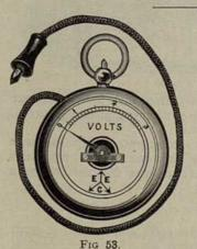
Suitable for testing separate cells or a number of cells in series.
