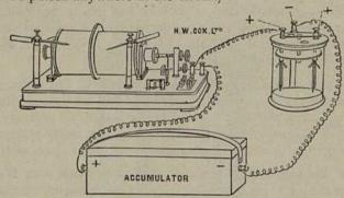
II. Electrolytic Break working off the mains.
