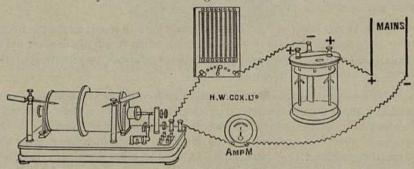
III. Showing connections when working from mains with Electrolytic and mercury interruptor in series with Rheostat and Ampere meter; (in this case the platinums on the coil are separated, but if the Mercury
