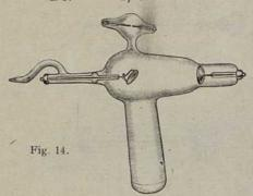
This Tube is made of glass which is opaque to the X-Rays, and does not allow them to pass effectively. They pass in abundance, however, through the window at the end of the projection, and can easily be concentrated upon any desired spot, so that the necessity for screening the healthy tissues while treating diseased parts, is obviated.
