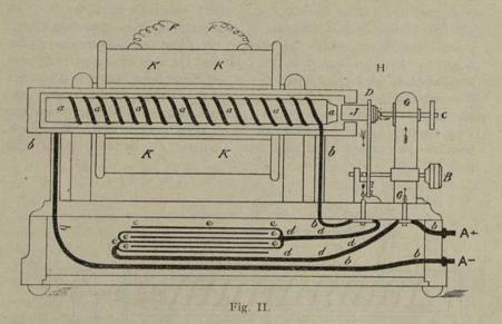
The device by which the primary current is thus interrupted is shown at Figs. II. and III. In Fig. II. the primary circuit is closed. The current passes from the positive terminal (+) up the metal pillar (G), by way of the platinum points (H) to the hammer or contact breaker (J), down the spring of the hammer (D), and thence by way of the primary circuit (bb), round the core (aa), and back to the negative terminal (-).
