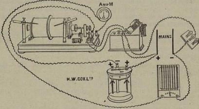
Interruptor is not used the platinums must be screwed up tight to each other). The diagram also shows a lamp resistance for working the motor of the Mercury Interruptor. The motor can, if desired, be driven from Accumulators.
