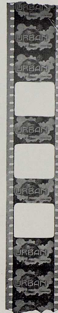
Small piece of film after three intentional firings in the Urban-Joy Gate.
